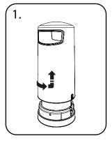
To open, turn bin body anticlockwise, and lift the bin body over the liner.
