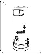
To close, lift bin body over the liner and lower to rest on plinth, turn clockwise until the bin body engages with the plinth track way and locks with a click.
