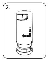
To close, lift bin body over the liner and lower to rest on plinth, turn clockwise until the bin body engages with the plinth track way.
