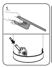
To open, ensure the illustration on the key is uppermost. Then insert the key all the way into the lock. (Do not turn the key.) This will release the locking mechanism.
