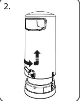
With the key still in position, turn bin body anti-clockwise, and lift the bin body over the liner.
