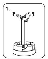
Release the sack retention bands by lifting up.
