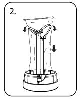
Insert the sack, fold over the sack retention bands and push the sack bands back into position.
